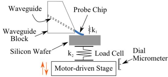
Figure 7. Mechanical test setup used to determine the effective spring constant of the probe tip.
