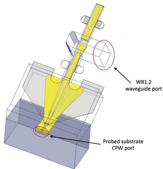
Figure 5. Full HFSS model of probe, port 1 - WR-1.2 waveguide, port 2 - probed substrate CPW.
