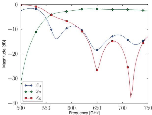
Figure 11. Simulated s-parameters of the WR-1.2 probe in the WR-1.5 frequency band
