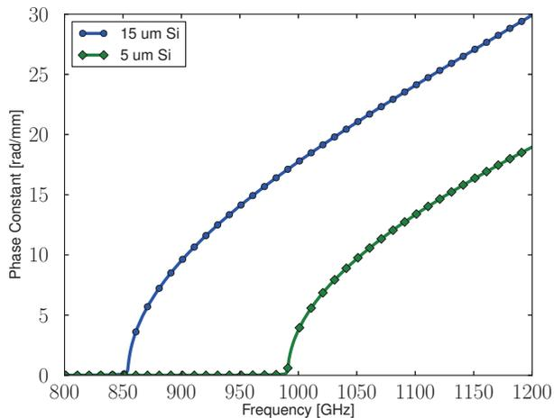
Figure 3. Cutoff frequency of first spurious mode in the coaxial channel for 15μm and 5μm Si substrates.
