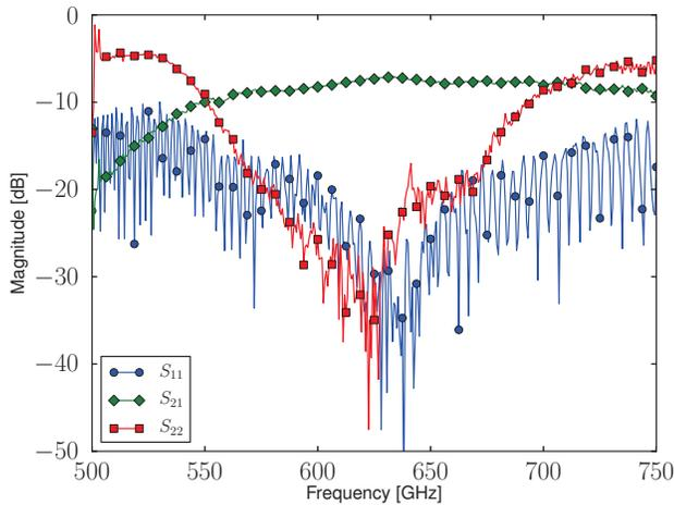
Figure 10. Measured S-parameters of the WR-1.2 probe in the WR-1.5 band.
