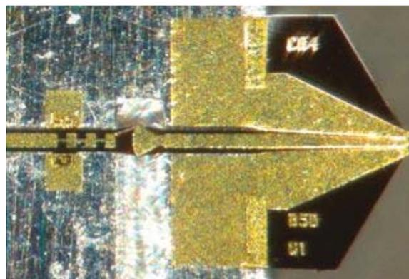
Figure 2. Micrograph of a WR-1.2 probe chip mounted in one half of the split-block waveguide housing, prior to being clamped in place. The E-plane probe is seen suspended over the waveguide channel.
