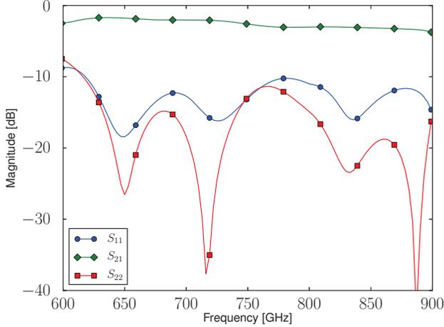
Figure 6. Simulated S-parameters of the WR-1.2 probe
