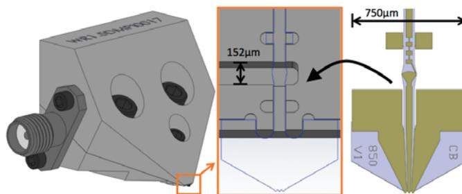
Figure 1. Self-aligned drop-in assembly process for micromachined on-wafer probe. The WR-1.2 waveguide channel height is 152  $\mu\text{m}$ .
