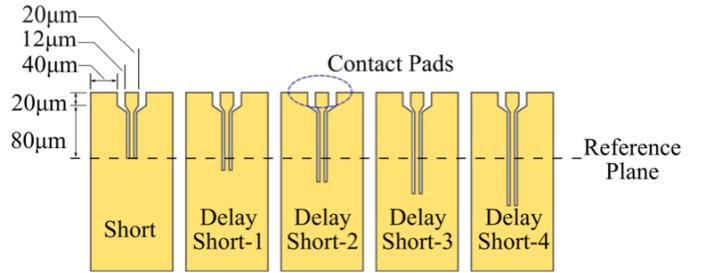
Figure 9. Layout of the CPW calibration standards. The CPW is 5/10/5  $\mu\text{m}$ .
