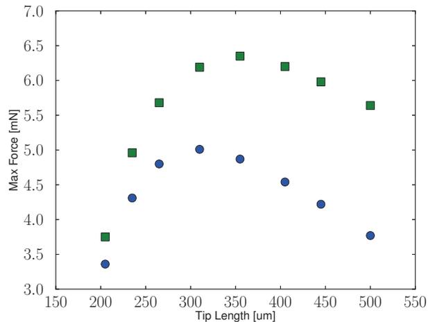
Figure 4. Maximum force generated at probe tip for various tip geometries. The circle markers indicate a 750 μm wide and the square markers indicate a 1500 μm wide tip.
